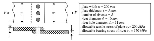
If the plates are to be designed to avoid tearing failure, the maximum permissible load P in kN is
